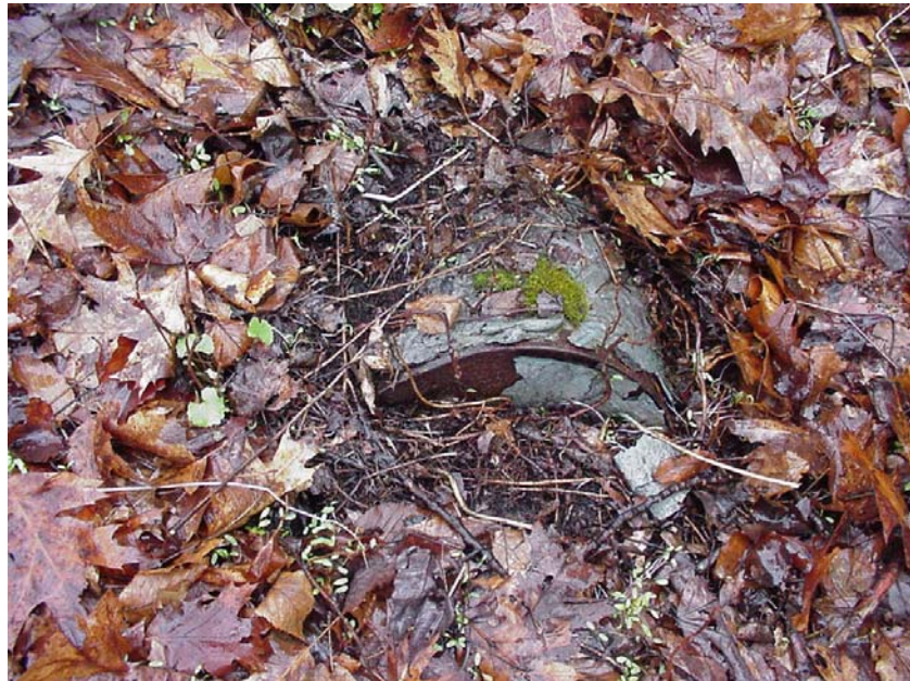
Photograph 6: Buried 55-gallons metal drum
