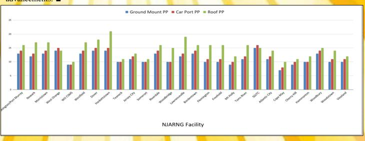
Payback periods for NJARNG facilities for ground-mounted solar panels (blue), car port panels (red), and roof-mounted solar panels (green)
