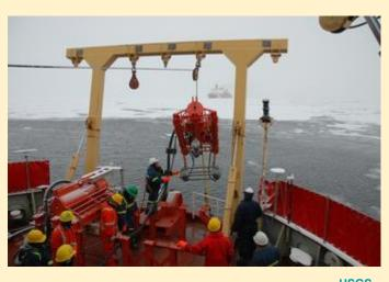
USGS An air cannon, also known as an air gun, being lowered into the water for the purpose offshore seismic exploration to locate oil and gas deep below the ocean floor.
