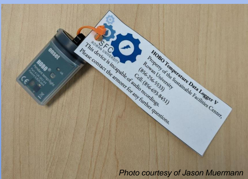
Figure 1. HOBO meter placed during the Somerset Readiness Center energy audit.
